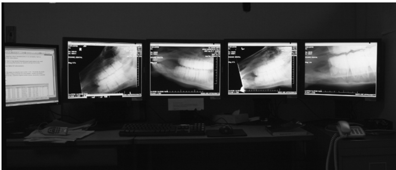
FIG. 2. Primary large animal radiograph review station. Four, 3 MP, medical grade monochrome (GSDF calibrated) are positioned in landscape mode in a semi-circular configuration. An additional color monitor enables the simultaneous viewing of other programs such as the web based Hospital Information System (HIS). To run five monitors, two additional graphics cards must be added to the computer. GSDF, grayscale display function standard.
